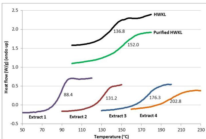
Figure 1: Differences in glass transition for a hardwood kraft lignin purified and sequentially solvent extracted.
