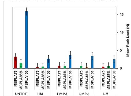
**Figure 2:** Change in peak load (tensile strength) of PLA mulches over 10 wk of soil burial. MB-PLA/PHA of 75%, 85% and 100% showed a decrease in peak load for all the treatments. SB-PLA showed no decrease in peak load for all the treatments, 10 & 30 wk (not shown).
