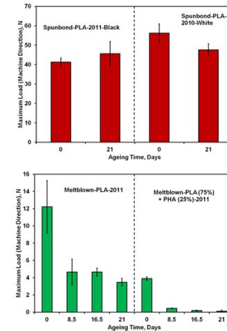
**Figure 4:** Effect of weatherometry treatment on tensile strength (breaking load)
