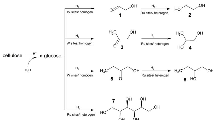
**Figure 1.** Reaction scheme of the hydrogenolysis of cellulose over Ru/W/AC with the main products: glycolaldehyde 1, ethylene glycol 2, 1-hydroxy-2-propanone 3, propylene glycol 4, 1-hydroxy-2-butanone 5, 1,2-butanediol 6, sorbitol 7.
